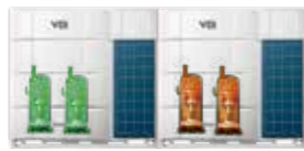
Continue operating in case of failure of one unit
