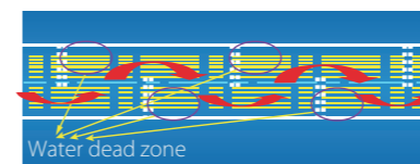
Flat baffle plate
